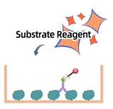
4、Add 100μL Substrate Reagent. Incubate for 15 min at 37°C
